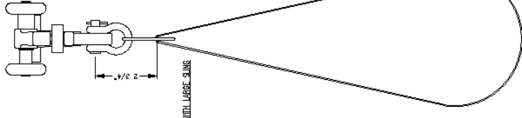
20084 EDL-8 FESTOON TROLLEY WITH LARGE SLING
